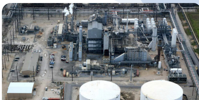
Aerial view of Air Products' existing steam methane reforming facility at Port Arthur, Texas, with new carbon-capture units and central co-gen and CO 2 product compressor
